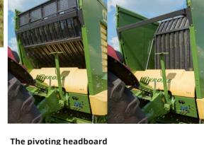
The RX 400 and RX 430 feature a headboard that pivots as a complete unit. When the machine is being filled by the forage harvester, this headboard pivots forward (A) for smooth and convenient filling without losses. When the machine is collecting grass with the pick-up, the headboard moves into a nearly vertical position (B) and pivots towards the tractor (A) to expand the capacity when the load area is full.
