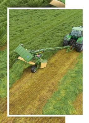
The trailed EasyCut disc mower with side-mounted drawbar and swivel gearbox gives you the flexibility of mowing round and round without lifting the machine out of work, without reversing and without ever stopping. The short drawbar makes for a compact combination that gives excellent rides and caster.
