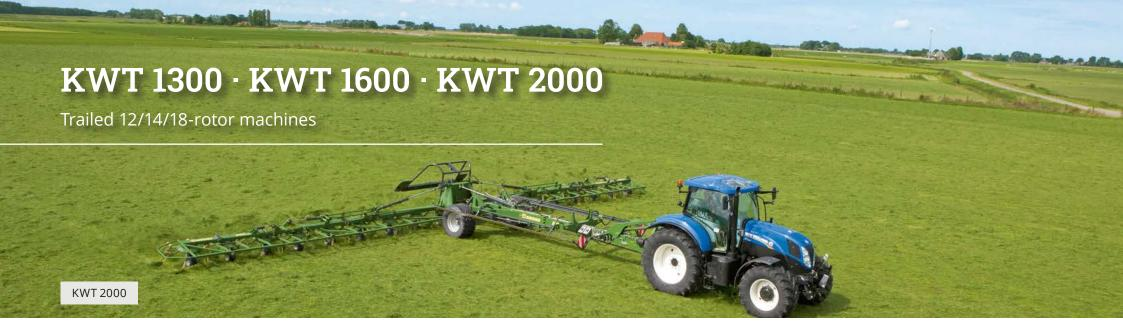
Making quality forage not only requires high-capacity mowers but also the right tedder. In terms of work rates, the KWT 1300, 1600 or 2000 is the perfect match for a high-capacity mower combination. It allows you to do the tedding pass in parallel with the mowing pass to achieve uniform wilts.
