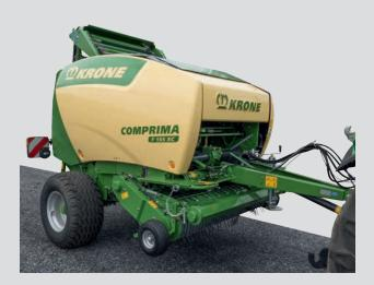
to their uncluttered build and design. It can unload bales of different diameters and compacts from the outside to the inside; with larger bale diameters, it leaves only a very small soft core. Thus, it achieves high bale weights.
